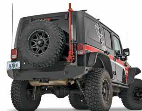
Elite Rear Bumper shown with optional off-road jack mount
