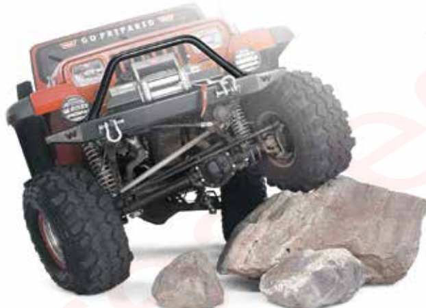
YJ WRANGLER with Front Rock Crawler Bumper, grille guard tube, and winch mounting plate
